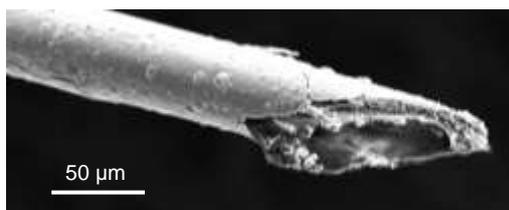
Fig. 4 SEM image of sharpened hollow microneedle made of stacked Ti and Parylene film.
